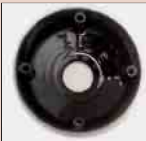
Interior coating of a diffuser
